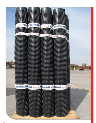
The naps of Fondaline resist against compressions even higher than 250 kN/m<sup>2</sup> keeping continuously an air gap of 5,5 l/sqm between the walls or floors of the building and itself. This space is big enough for the drainage of the rain or ground water, as well as for the evaporation of humidity if supported with a suitable system of ventilation.
