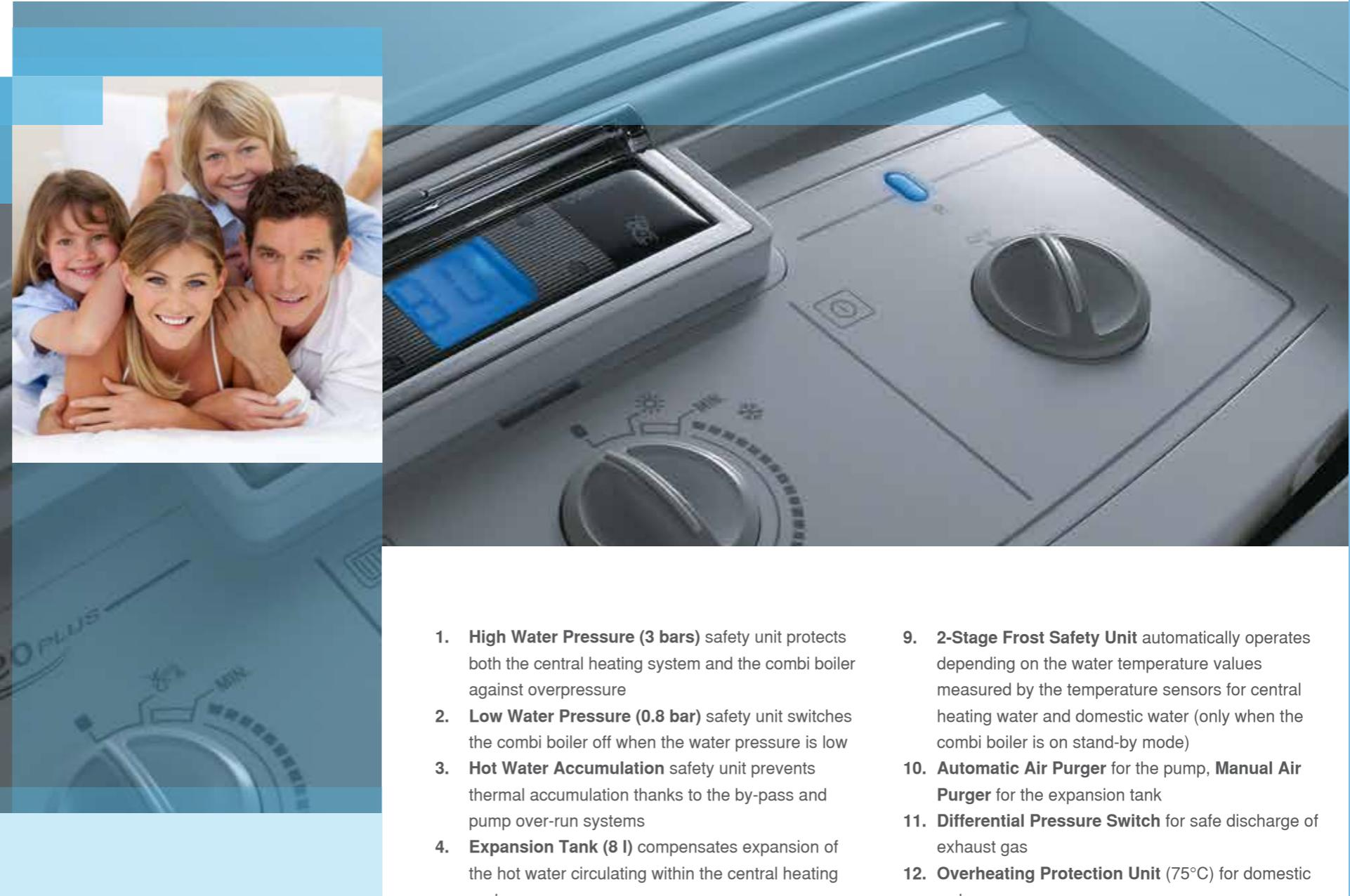
1. **High Water Pressure (3 bars)** safety unit protects both the central heating system and the combi boiler against overpressure
